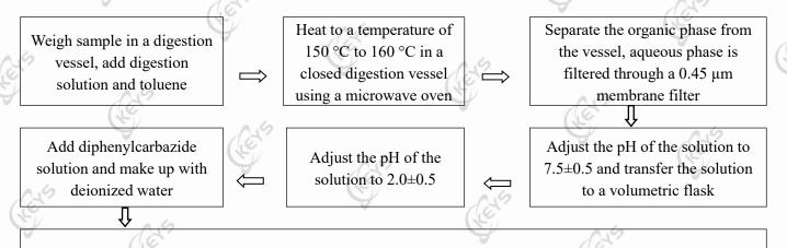
Analyze the mixture by using UV-Vis Spectrophotometer with wavelength set at 540 nm
